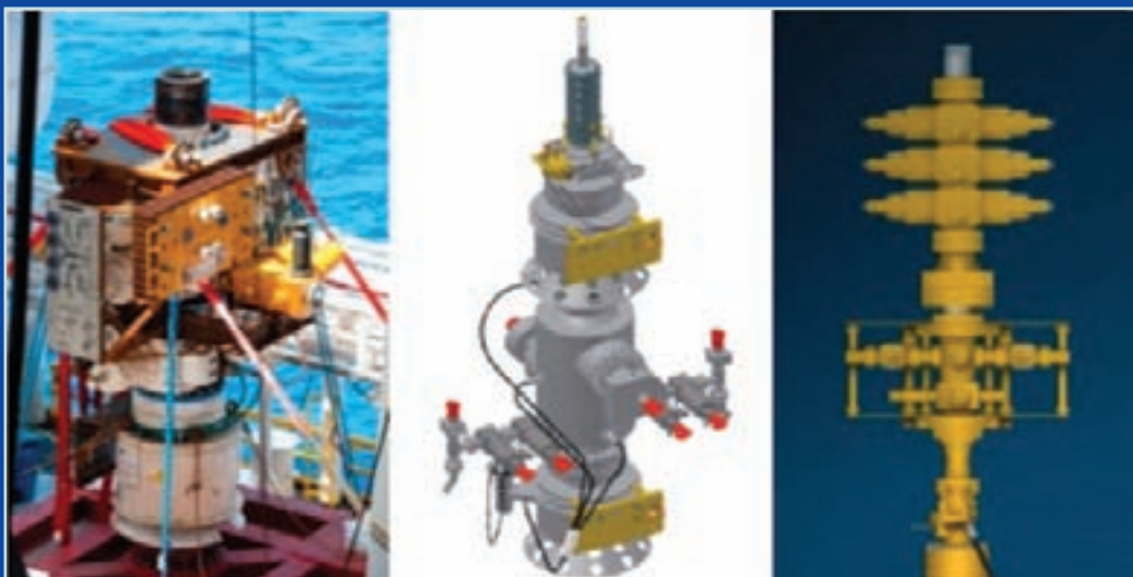
Figure 6.1 Custom-made Capping Stacks (left Flange Stack used on Macondo, Middle OSPRAG, Right MWCS)
