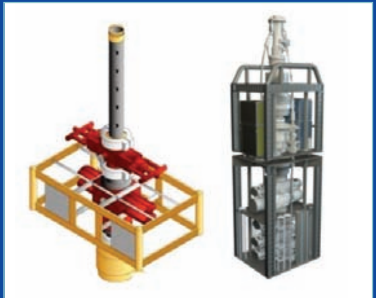
Figure 6.4 BOP Configurations - Small BOP with RAMS (Left), Full Size BOP (Right)
